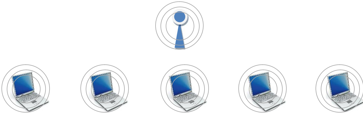
Figure 2-1: General setup of a wireless network, illustrating that both the AP and the end devices emit RF EMFs.
